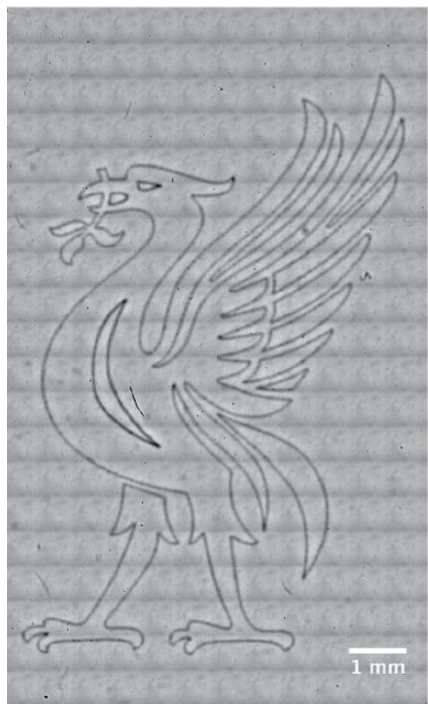
Figure 0-6. Demonstrative refractive index gradient examples. Stitched DIC microscope images of (a) direct laser write of a bird pattern, (b) projection mask lithography of a 1-inch diameter Fresnel lens.
