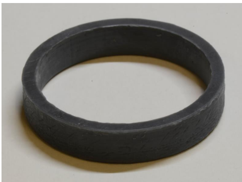
Figure 0-5. Close-up photograph of the ring showing the Elvish inscription was faithfully captured during the 3D print of the thiol-ene HDT-DAT thermoplastic resin.
