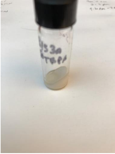
Figure S1. Loss of transparency of precursor resins at higher TBPA loadings (50 wt%)
