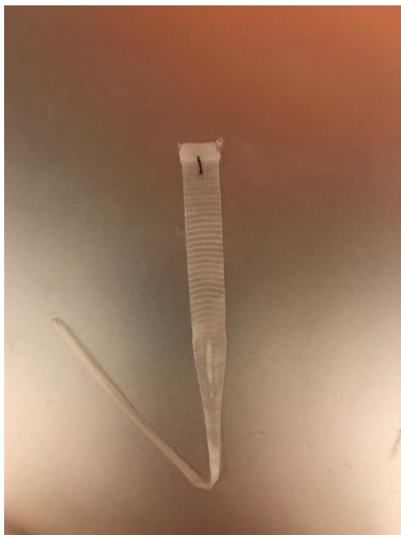
Figure 0-17. Photograph of one end of a HDT-DAT ASTM D368 Type V dogbone strained to failure with visible periodic striations of opaque and translucent regions.
