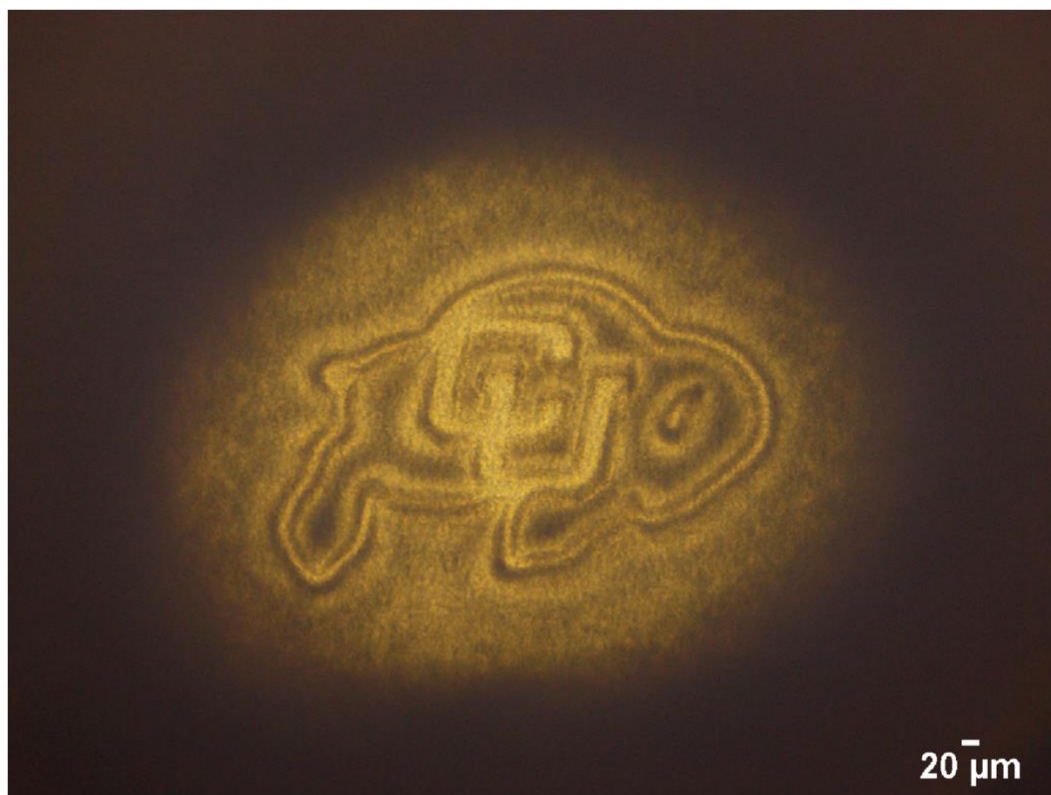
Figure 0-1. A CU buffalo is imaged patterned on a neat HDT-DAT thiol-ene resin using a commercial DLP attached to a polarized microscope. Feature sizes on the order of several microns can be discerned with some over-cure observed.
