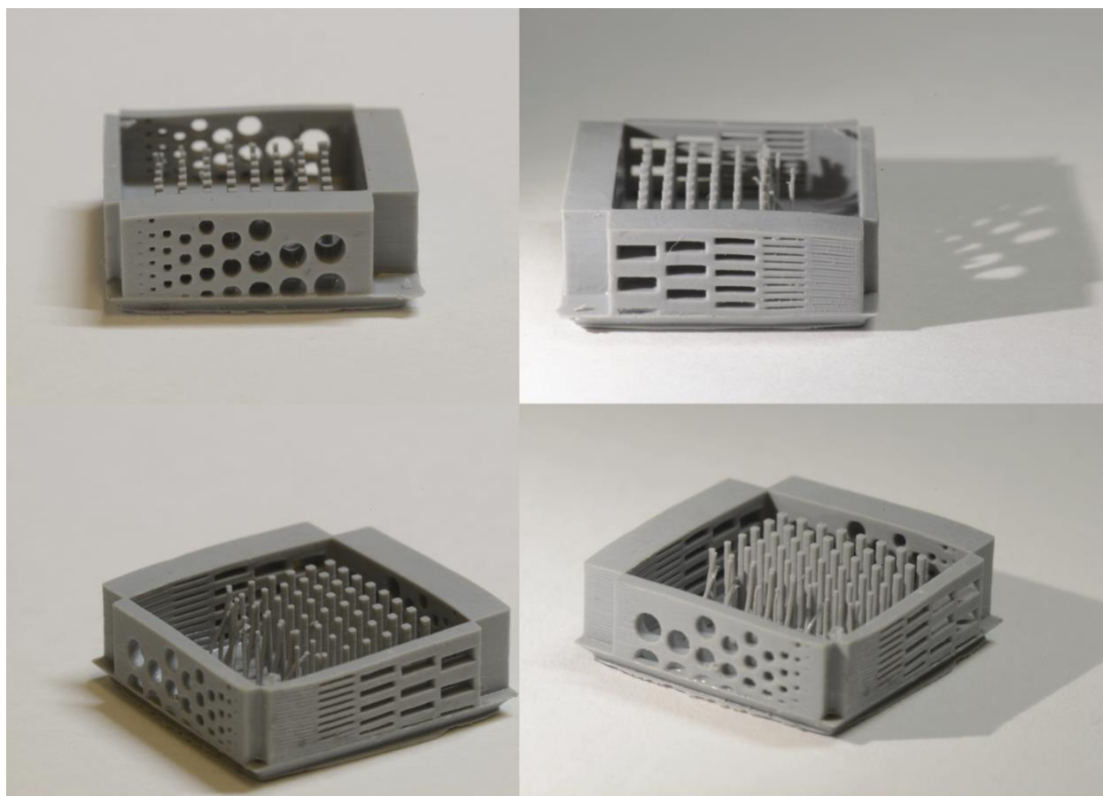
Figure 0-3. Photographs of a QC 3D print at multiple angles showing the high spatial resolutions achieved with both positive and negative features.
