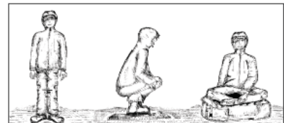
Fig. 4 Lightning positions: Put your feet together to significantly reduce the effects of ground current. If you have a foam pad to stand on or a pack to sit on, get on it. Crouch or sit to slightly reduce the effects of side flash and upward leaders.
