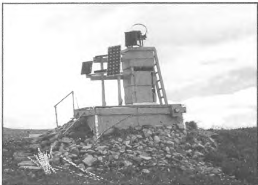
Subnivean Lab (built in 1993) in the Saddle on Niwot Ridge collects data on snowmelt for the Niwot Ridge LTER program. (J. Kindig)
