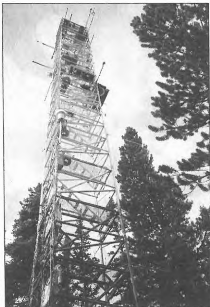
Instruments in this 30-meter tower measure the flux of atmospheric gases. (J. Kindig)
