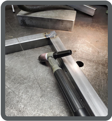
Two frame bars in the process of being welded together
