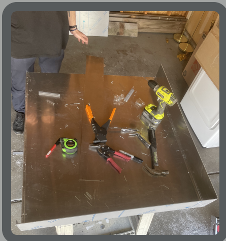
The base tub in the process of being riveted together
