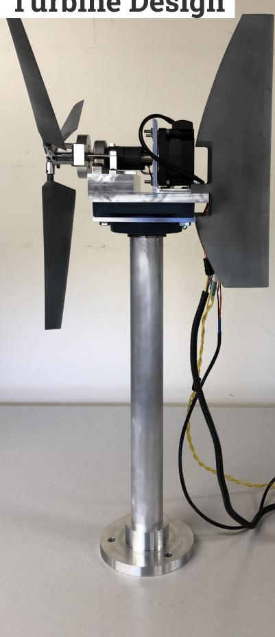
A scale turbine was designed to fulfill competition performance requirements and reliably capture the wind to develop a steady power curve.
