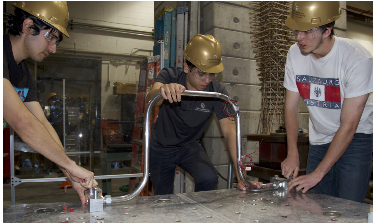
Isaiah, Nestor, and Joe securing the expansion loop to the CIEST vibration table
