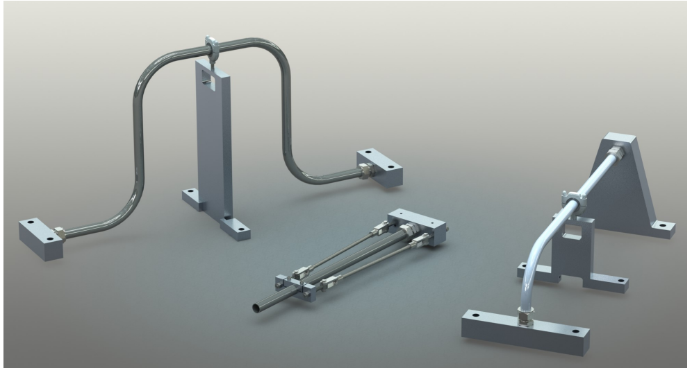
All 3 systems: Expansion loop (left), Cantilever (middle), and 90 degree bend (right) rendered in SolidWorks with restraints applied
