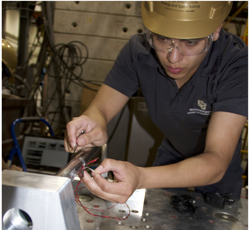
Nestor adjusting a strain gage on the 90 degree bend system just before testing on CIEST table
