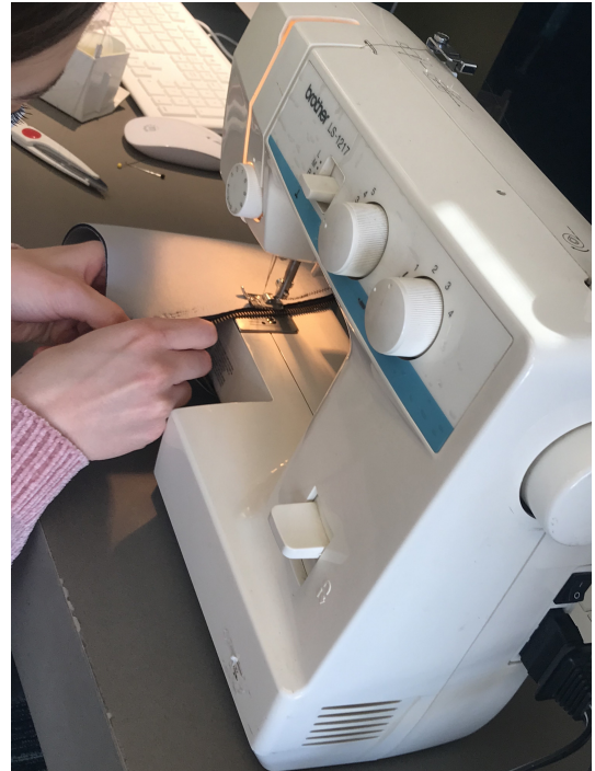
Figure 17. Sewing the neoprene sleeve
