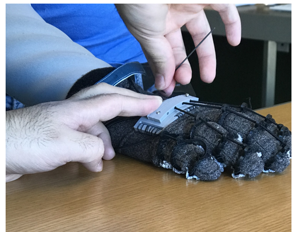
Figure 9. Adjusting shock cords with screw tightening system
