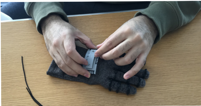
Figure 16. Assembling the back of the hand plate
