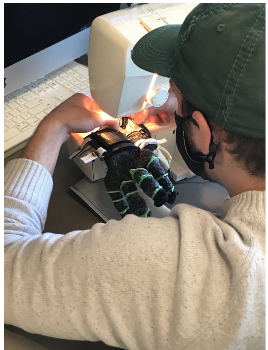
Figure 18. Sewing components to the first prototype
