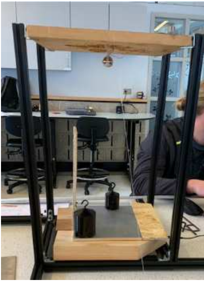
Figure 2: Early stage test fixture. A ball bearing is dropped from a constant height onto the metal plate below.
