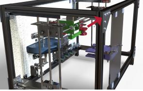
Transport sample across working volume via 2-axis gantry and swing arm
