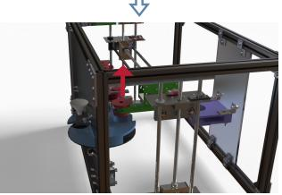
Pick up sample using 2-axis gantry and swing arm
