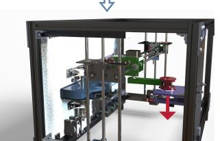
Drop off sample at instrumentation suite by lowering the vial into place
