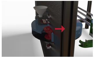
Rotate turntable to shear off excess sample and bring vial inside the lander
