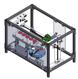
The final system design is shown above. The exploded version below highlights each subassembly and its purpose. Critical components are highlighted in color for clarity.
