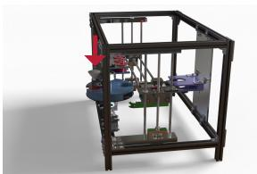
Receive sample in funnel and fill vial in turntable below
