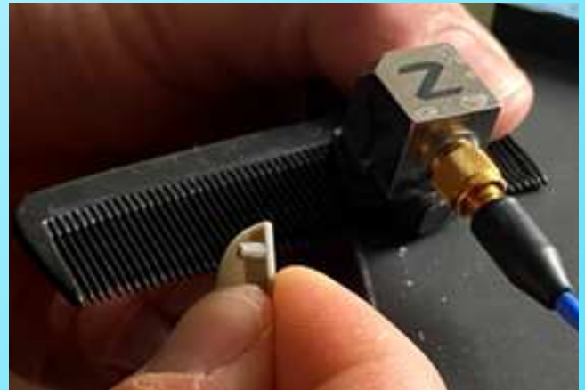
Figure 3: Accelerometer Mounted to a Comb to Measure Vibrations Caused by Plucking Teeth.
