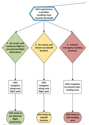
Flight scenario outcomes once the drone is in flight and experiences a weather condition that exceeds a threshold
