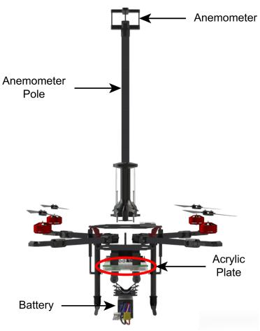
An exploded view of the UAV and FMS assembly
