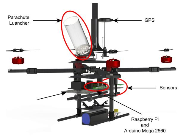
A close-up view of the UAV and FMS assembly
