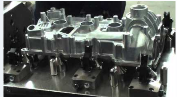
Thin-walled part gripped by its fixture
