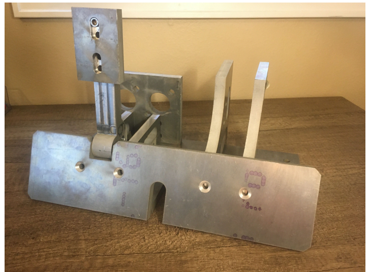
Figure 32: Partial pedal assembly with brake pedal shown
