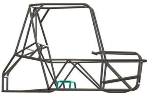
Figure 2: Chassis with Raised Seat Structure Highlighted in Blue
