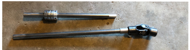
Figure 33: Top: Upper steering column with bearings and retention collars Bottom: Lower steering column with U-joint
