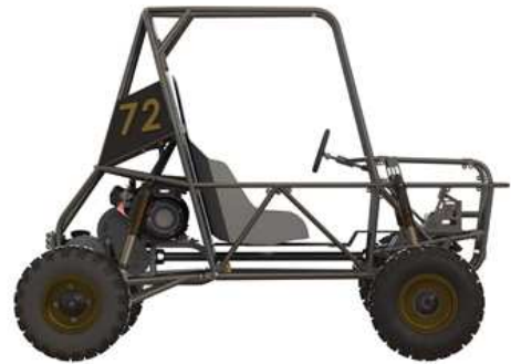
Figure 3: Chassis with False Floor and Center Driveshaft
