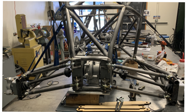
Figure 16: Rear suspension during fitment and welding process
