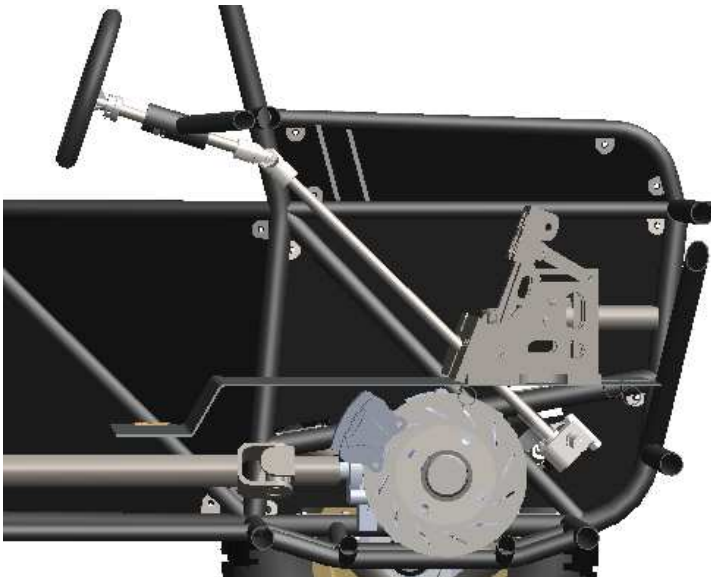
Figure 26: Section view of the vehicle toe-box complete with front brakes, pedal assembly and steering system
