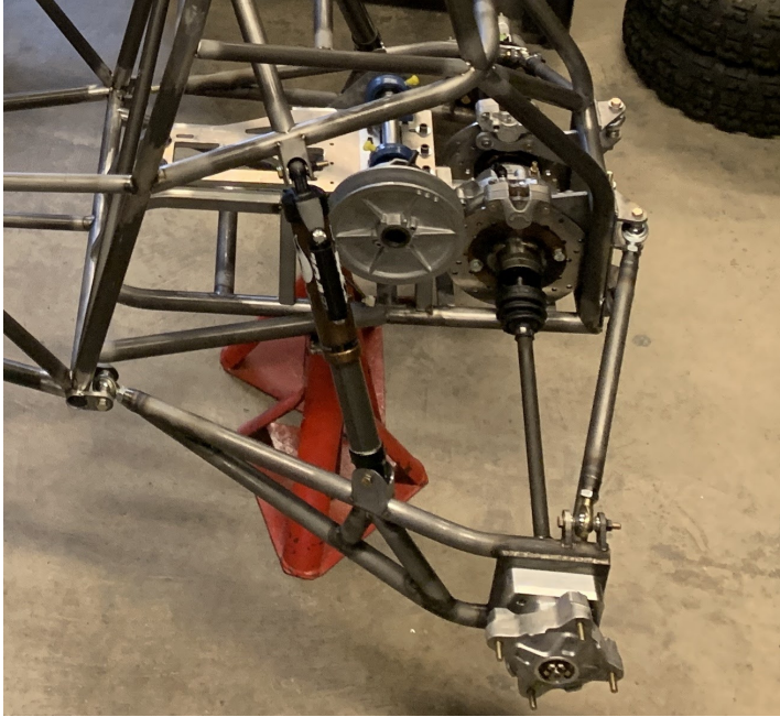
Figure 15: Left hand suspension assembly as manufactured
