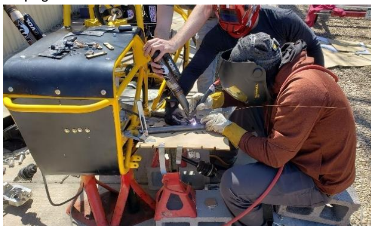
Figure 21. UCA fixtured in place during welding.
