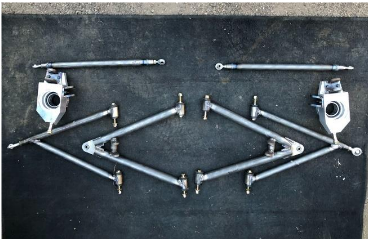
Figure 23. Redesigned Front suspension components including UCA, LCA, Steering Uprights, and Tie Rods
