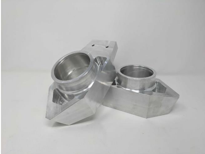
Figure 22. Redesigned Steering Uprights after CNC Milling Operations
