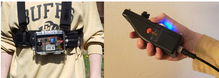
Figure 2: a) Final design of the skier belt with the communication box centered on the front of the belt. b) Final design of the guide controller with the emergency-stop button on the side of the device.
