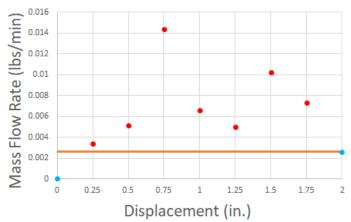
**Figure 5:** Correlation between displacement and the mass flow rate recorded at the no flow condition (no fluid) of the 1/2" CMF Coriolis Meter. Data was collected at a meter orientation of 90 degrees.
