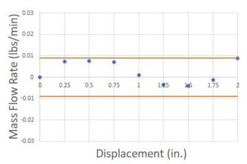
**Figure 6:** 1" F-Series Coriolis Meter - Correlation between displacement and the mass flow rate recorded at the no flow condition (no fluid). Data was collected at a meter orientation of 0 degrees.
