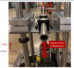
**Figure 1:** Bottle jack applies a vertical force on one side of the fixture, where the opposite end remains fixed.
