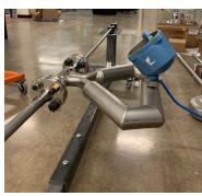
Figure 2: CMF meter in the 90 degree orientation.
