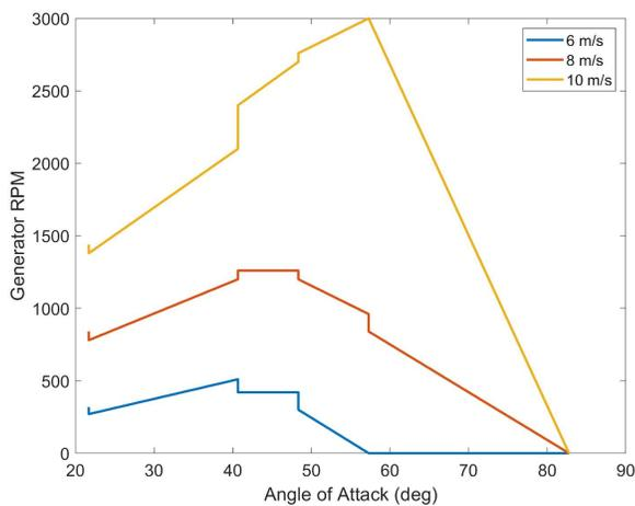
Primary data was collected to model the blade performance and pitch mechanism for the design of the active pitch control system as seen in the above graph.
