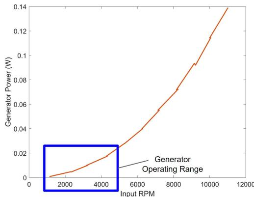
The results from this test are shown in the figure. This test was critical for defining the voltage and power outputs could be expected from the generator over a range of RPMs.
