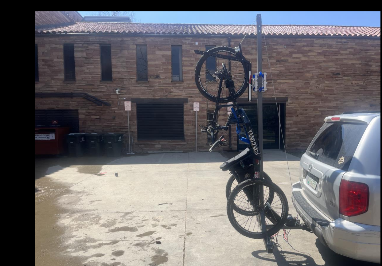
Step 4: Strap bottom wheels to horizontal collars with ratcheting straps
