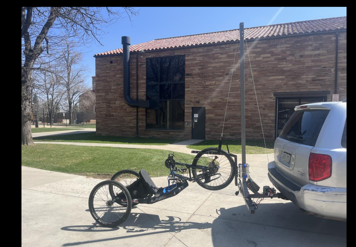
Step 2: Use remote to pull front wheel up until it reaches height of vertical collar and attach to the collar
