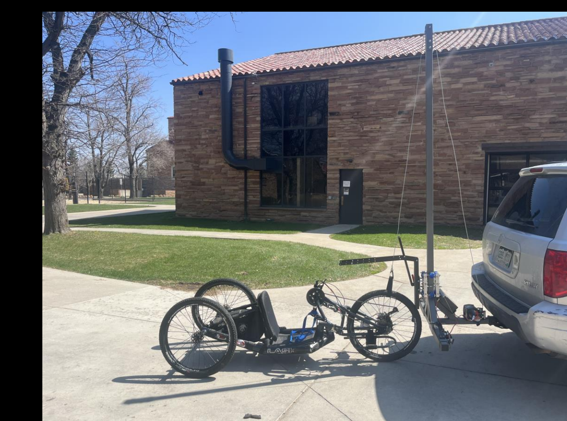
Step 1: Ride bike up with singular wheel to assembly Strap the winch through front wheel
