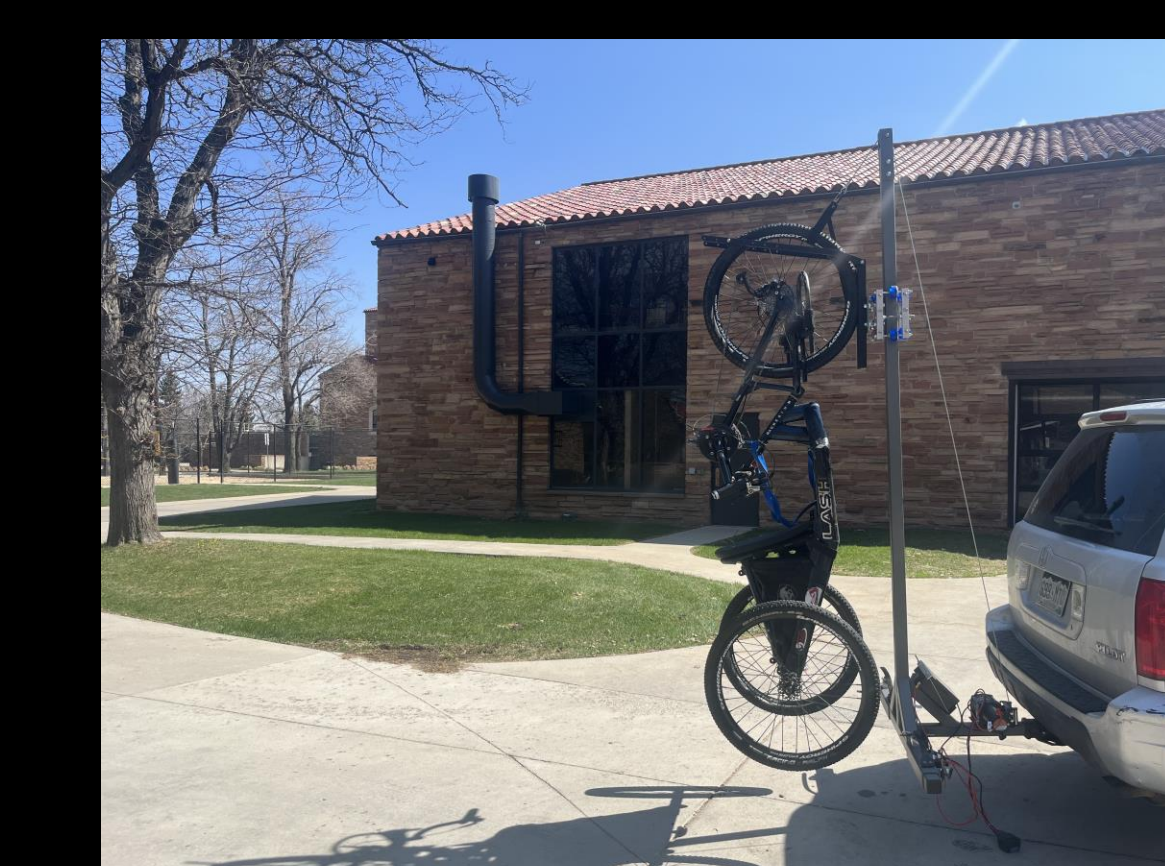
Step 3: Continue to raise bike until back wheels are off the ground
