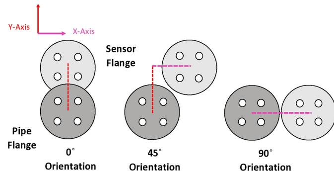
Figure 3: Pipe misalignment in respect to different angles in testing.
