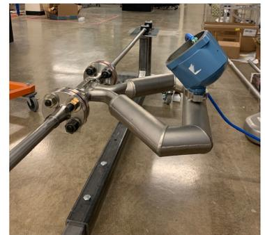
Figure 2: CMF meter in the 90 degree orientation.
