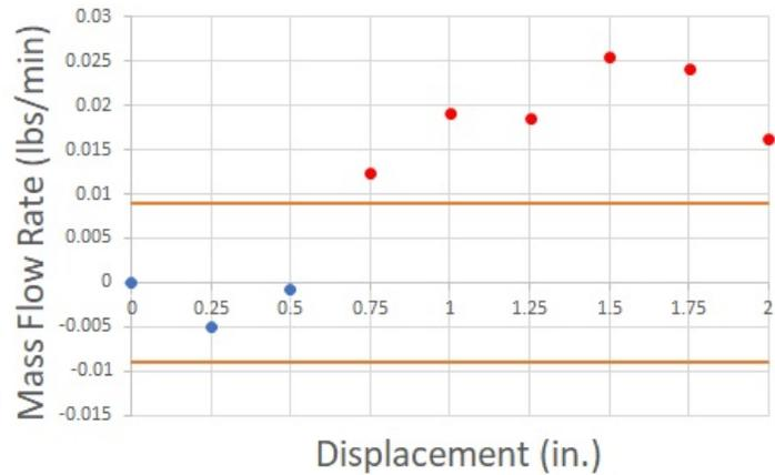
**Figure 4:** 1" F-Series Coriolis Meter - Correlation between displacement and the mass flow rate recorded at the no flow condition (no fluid). Data was collected at a meter orientation of 90 degrees.
