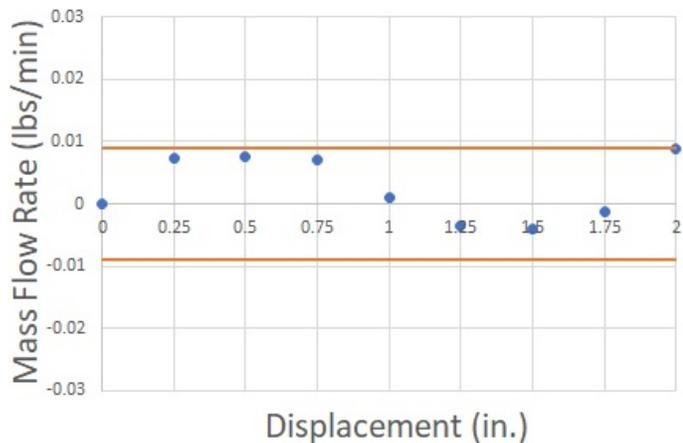
**Figure 6:** 1" F-Series Coriolis Meter - Correlation between displacement and the mass flow rate recorded at the no flow condition (no fluid). Data was collected at a meter orientation of 0 degrees.
