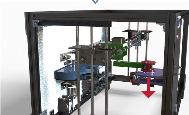
Drop off sample at instrumentation suite by lowering the vial into place
