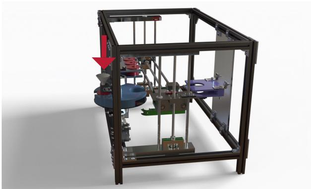
Receive sample in funnel and fill vial in turntable below
