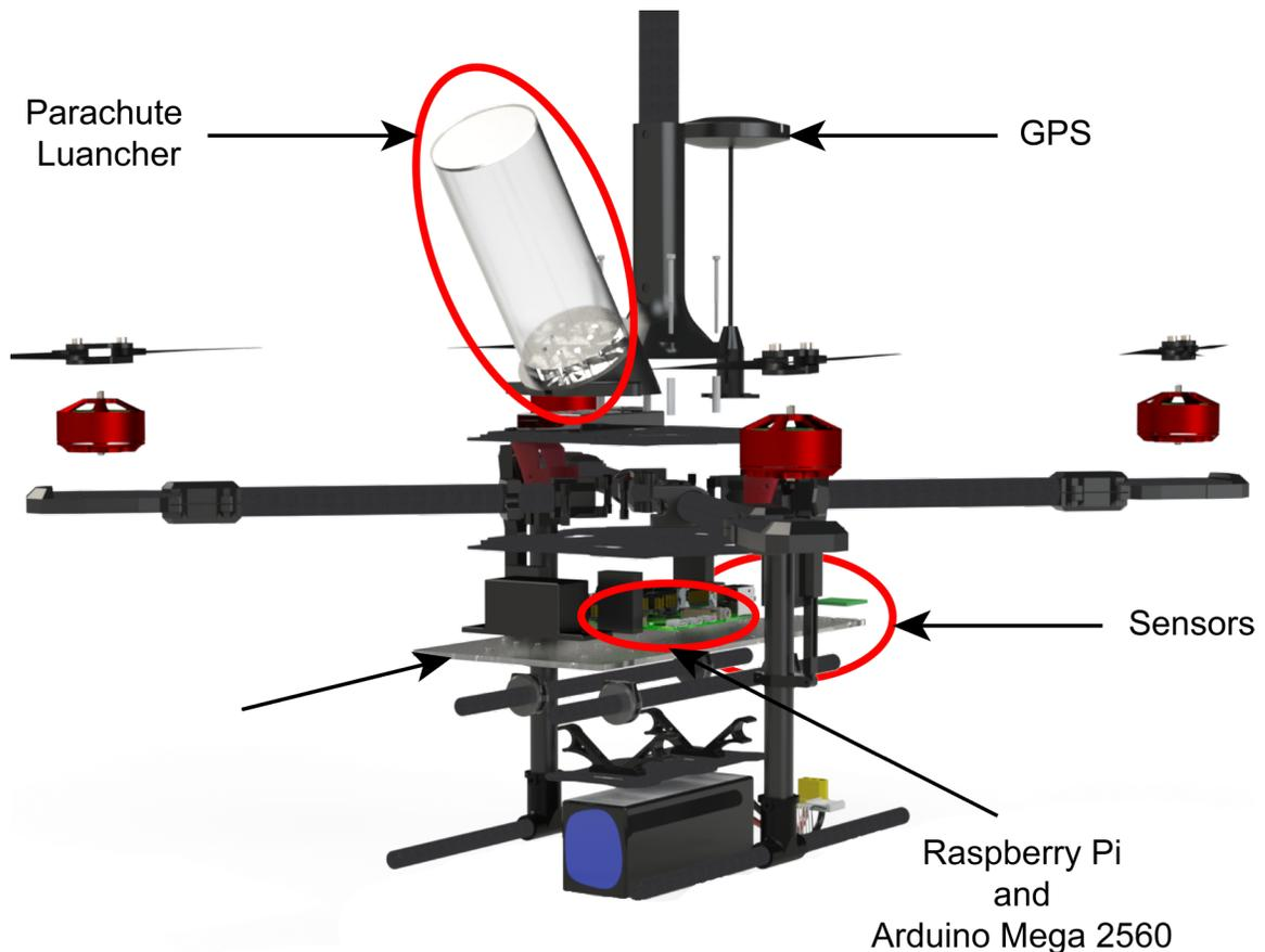
*A close-up view of the UAV and FMS assembly*
