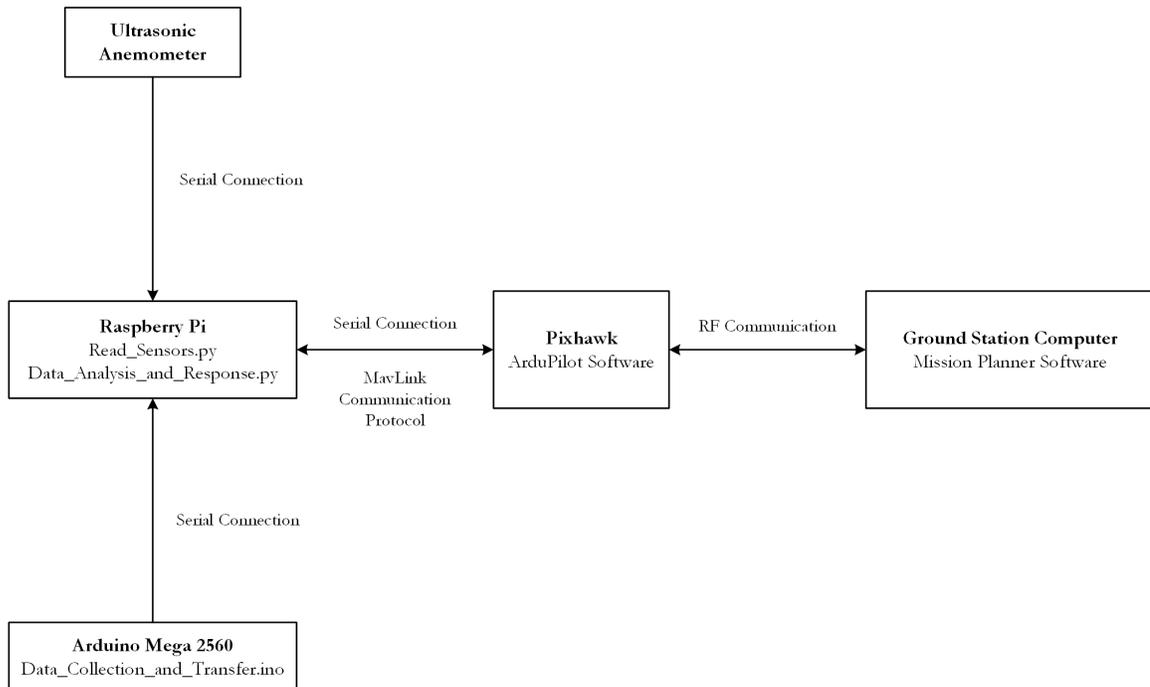
*A diagram showing the data flow and signal methods between components of the FMS*
