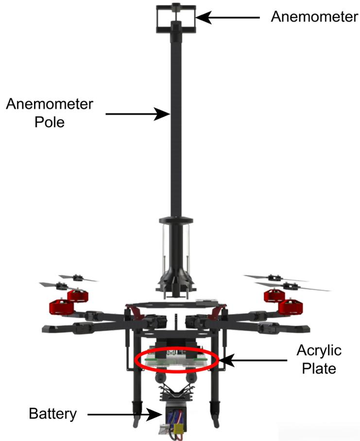
*An exploded view of the UAV and FMS assembly*
