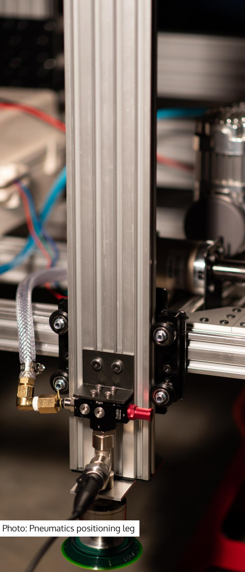
Photo: Pneumatics positioning leg
