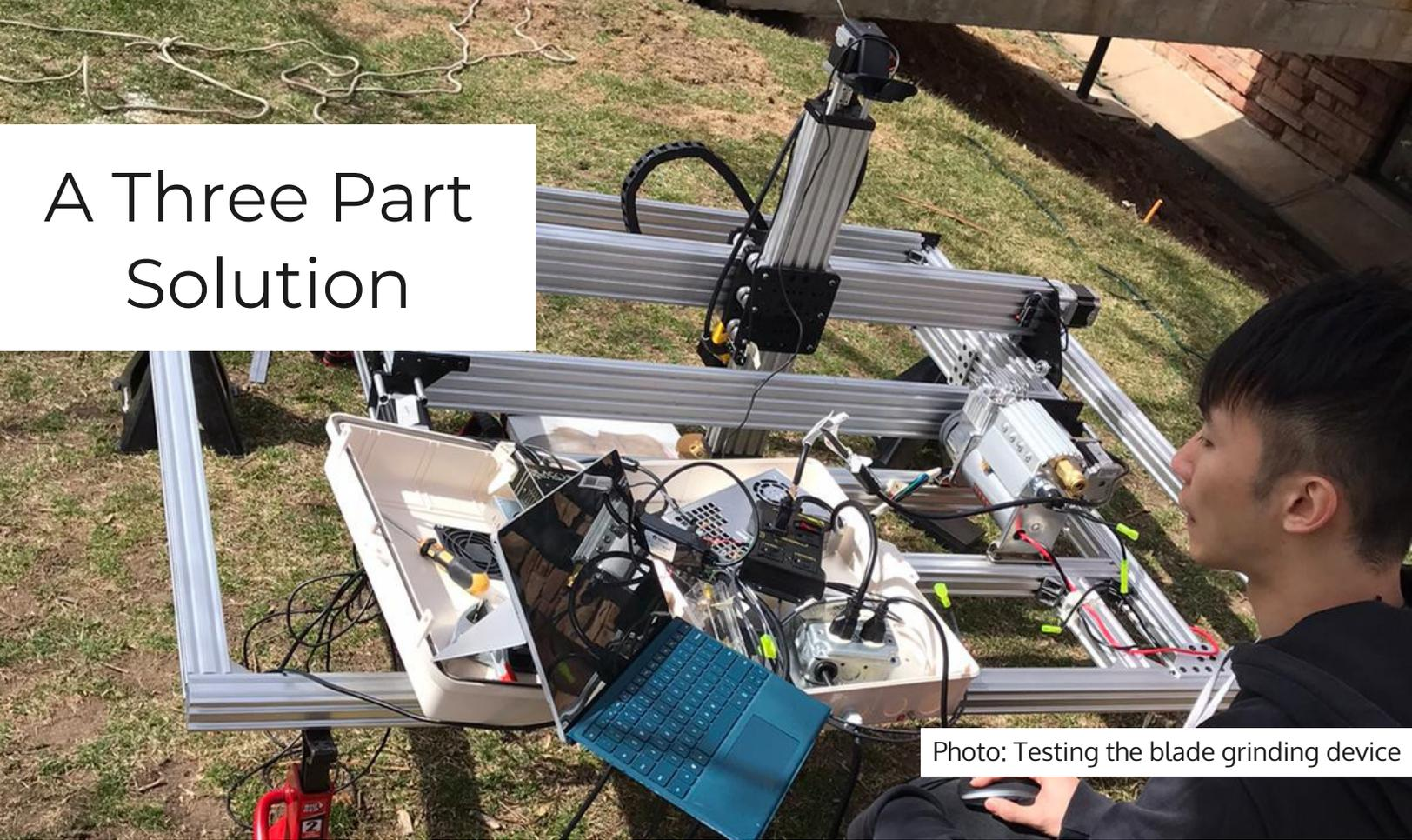
Photo: Testing the blade grinding device
