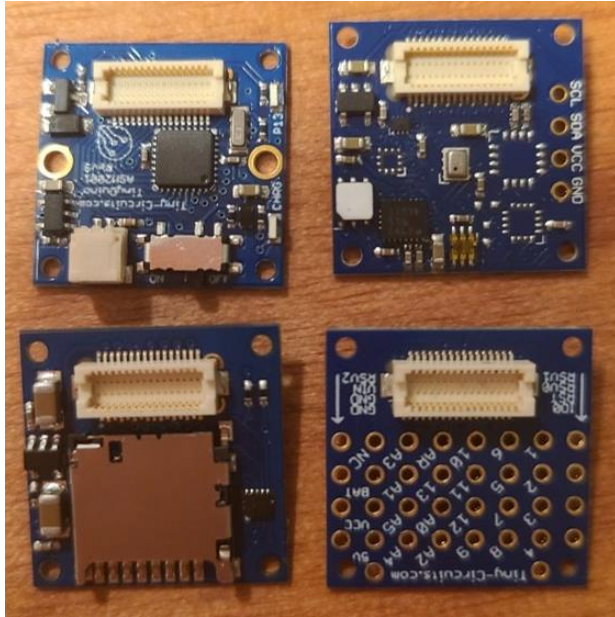
Figure 3: Tiny Circuits Breakout Boards. Going clockwise from the top right, there is an accelerometer/barometer, proto board, SD card writer, and microprocessor.
