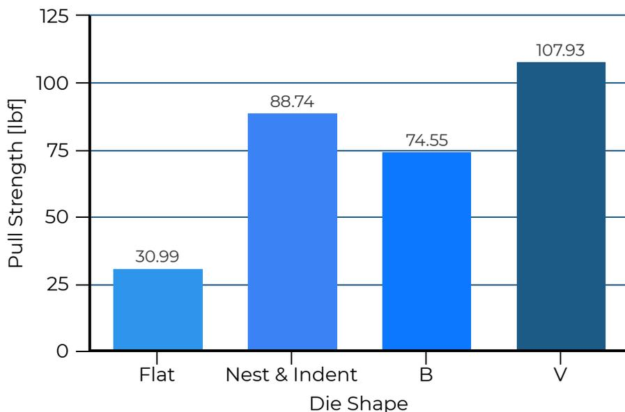
During the exploratory phase, each die shape was tested with the standard tube and no end modifications with crimp forces up to 6.5 kN.
