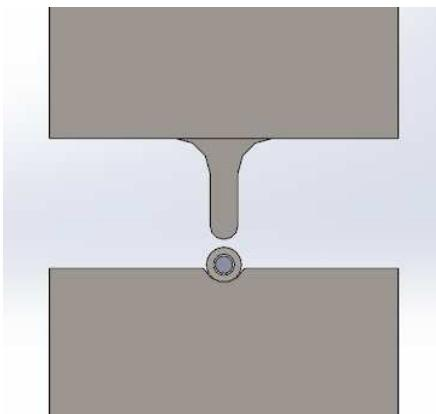
Cross-section view of Nest and Indent die shape with tube and cable for reference
