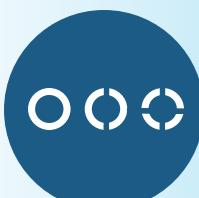
Tube End Modifications: Based on research the team did on "U-brackets", the team decided to investigate making small cuts on the end of the steel tubes. The idea behind this was that these cuts would not only change the way that the tube deformed when crimped, but also reduce the force required to crimp the tube. Three variations were tested; no slit, one slit, and two slits.
