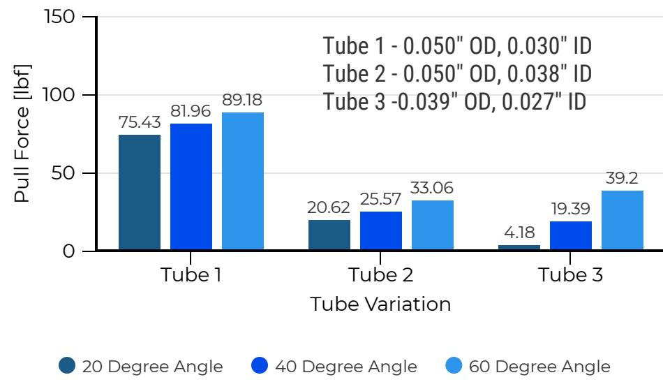
The team then tested each die shape variation at 3.5 kN and 4.5 kN, for this was the range the initial tested crimps began to pass the 60 lbf requirement.
