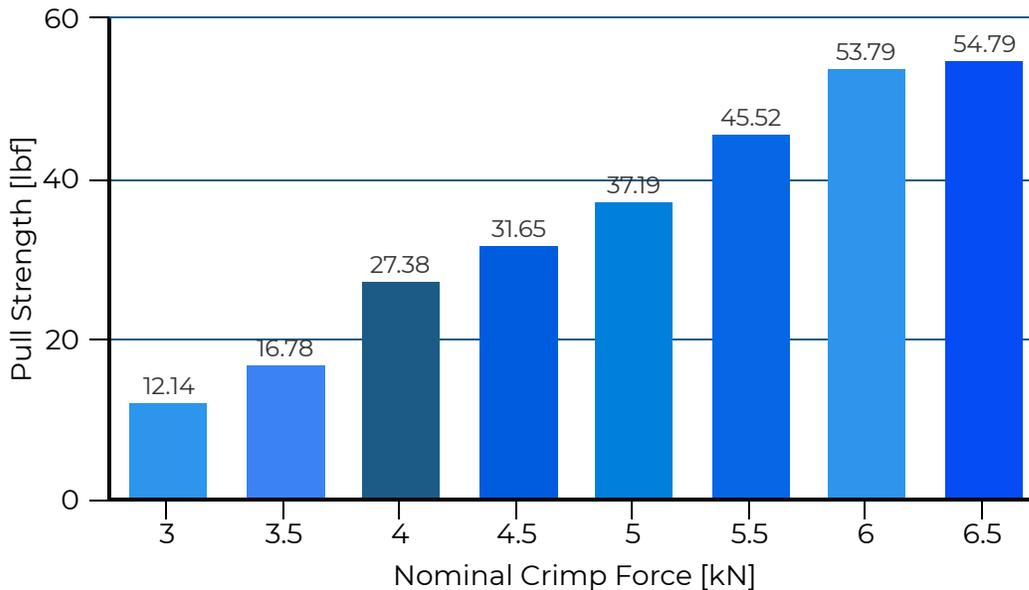
The V shape was first tested at the smallest clearance with no other variations applied yielding the results shown left. As shown, higher crimp forces yielded results closest to the passing crimp force of 60 lbf.
