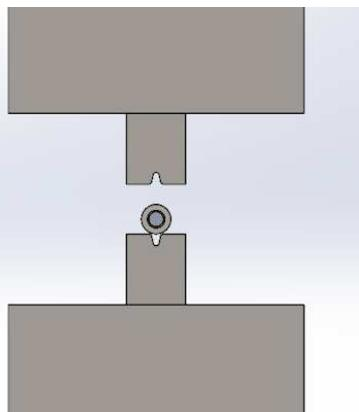
Cross-section view of V die shape with tube and cable for reference
