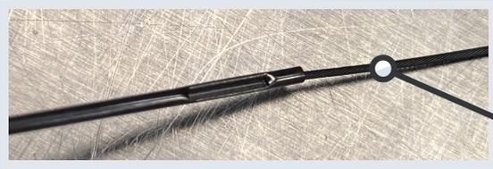
Multiple tungsten wires crimped to steel tubes fit inside the body of the device. Here is a crimped sample for reference.
