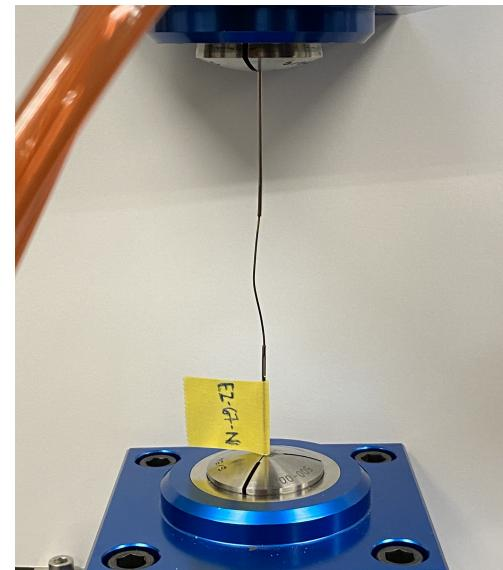
Instron Machine Crimped Sample Setup
