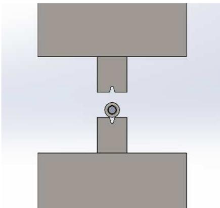
Cross-section view of V die shape with tube and cable for reference
