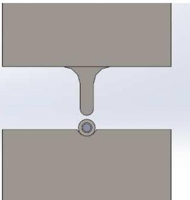
Cross-section view of Nest and Indent die shape with tube and cable for reference
