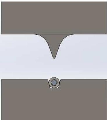
Cross-section view of B die shape with tube and cable for reference
