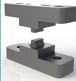
The V Die Shape showed promise after the initial testing. At 6.5 kN, the two larger variations, V2 and V3, both surpassed the 60 lbf pull strength requirement. Further testing is needed to complete the V shape analysis.
