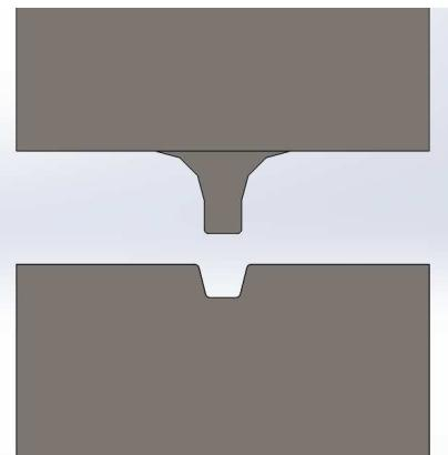
The Flat die shape was designed to have a flat rectangular shape with rounded corners to prevent damaging the tube. The upper die was designed with a width of 0.04" and the bottom die was designed to be exactly the same as the B-Crimp bottom die. The top die was wide enough to cover more than the width of the tungsten cable diameter (0.025") and the bottom die was small enough to maintain the crimped tubing area maximum diameter limit.
