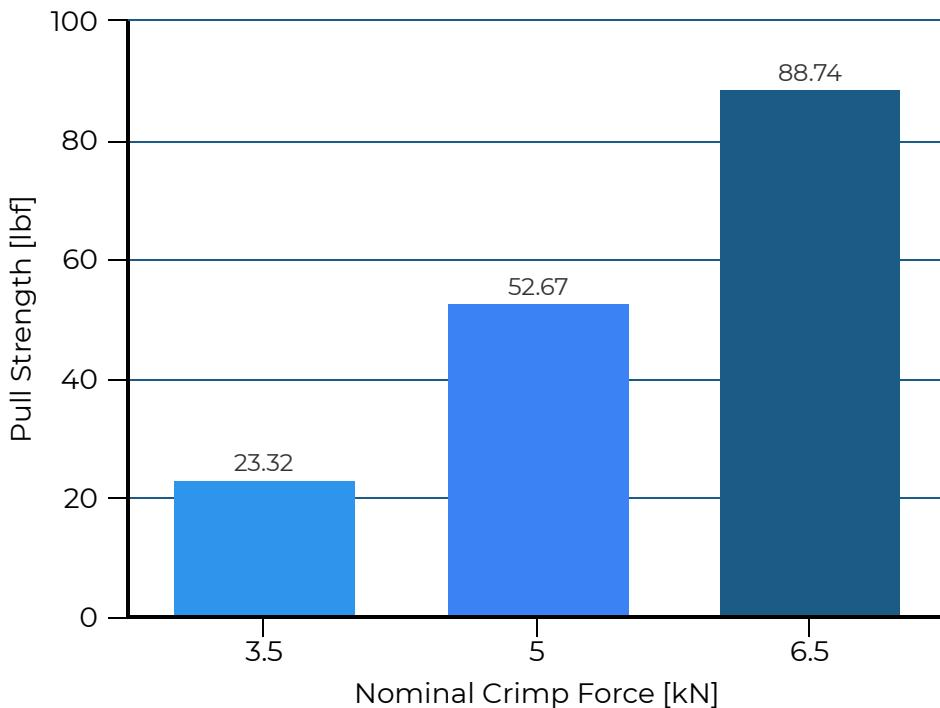
The Nest and Indent shape was only tested at three crimp forces. This allowed the team to develop an understanding of the die performance without testing a large number of samples.
