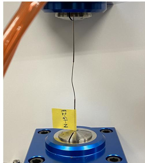
Instron Machine Crimped Sample Setup
