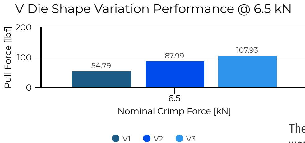
We then tested each die shape variation at 3.5 kN, 5 kN, and 6.5 kN to provide overall performance data on each variation in clearance distance. The 6.5 kN showed passing crimps for V2 and V3 as evidenced in the graph above.
