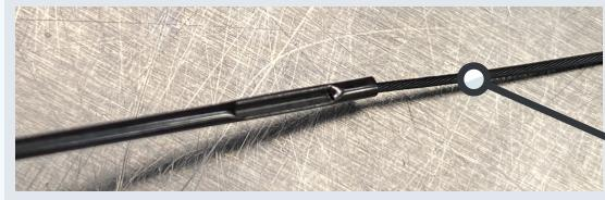
Multiple tungsten wires crimped to steel tubes fit inside the body of the device. Here is a crimped sample for reference.
