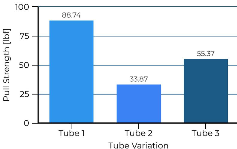
The Nest and Indent shape performs better with increased crimp forces when crimped with tube 1. Crimps performed on tube 2 and tube 3 did not yield successful crimps. Tube end modifications also did not yield successful crimps.
