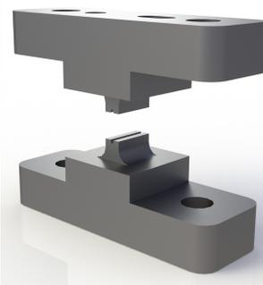
The V Die Shape showed promise after the initial testing. At 6.5 kN, the two larger variations, V2 and V3, both surpassed the 60 lbf pull strength requirement. Further testing is needed to complete the V shape analysis.
