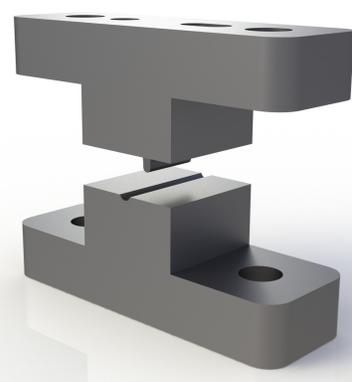
The Nest and Indent Die Shape produced successful crimps at 6.5 kN crimp forces. The tube variation showed Tube 1 as the best combination with this die shape.
