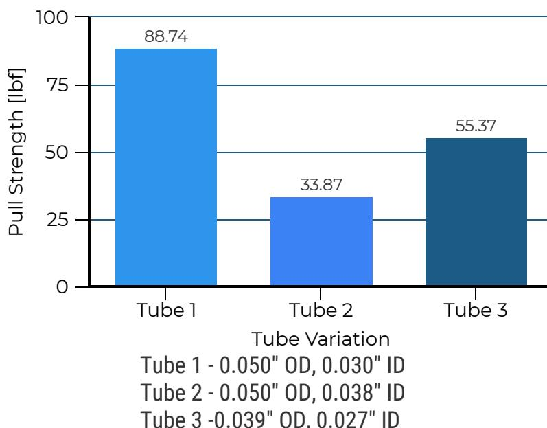
The Nest and Indent shape performs better with increased crimp forces when crimped with tube 1. Crimps performed on tube 2 and tube 3 did not yield successful crimps. Tube end modifications also did not yield successful crimps.
