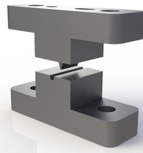
The B Die Shape produced successful crimps with crimp forces 4.5 kN and above. After comparative testing of the variations, the 60 degree angle paired with Tube 1 was the strongest combination.
