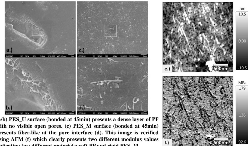
(a/b) PES\_U surface (bonded at 45min) presents a dense layer of PP with no visible open pores. (c) PES\_M surface (bonded at 45min) presents fiber-like at the pore interface (d). This image is verified using AFM (f) which clearly presents two different modulus values indicating two different materials: soft PP and rigid PES\_M.
