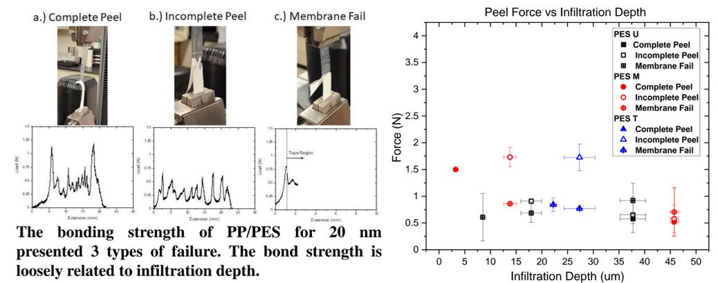
The bonding strength of PP/PES for 20 nm presented 3 types of failure. The bond strength is loosely related to infiltration depth.
