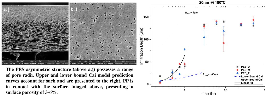
The PES asymmetric structure (above a.) possesses a range of pore radii. Upper and lower bound Cai model prediction curves account for such and are presented to the right. PP is in contact with the surface imaged above, presenting a surface porosity of 3-6%.
