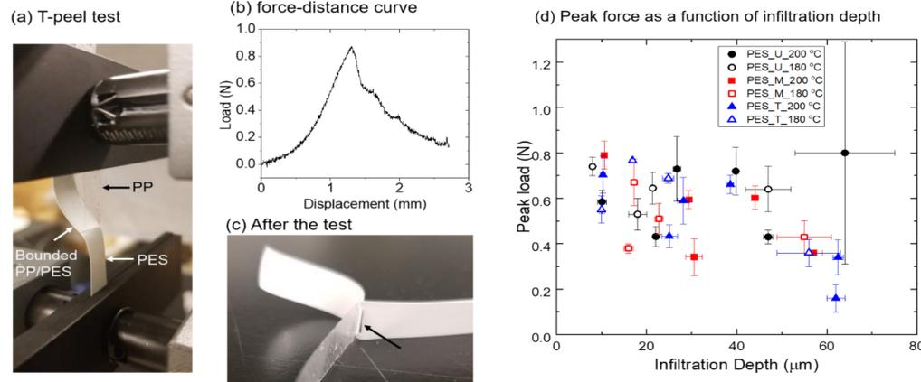
a) T-peel test set-up. b) the force distance curve representing the peak force achieved. c) image of membrane failure at the bonded interface. (d) Infiltration depth vs peak load achieved in (b)
