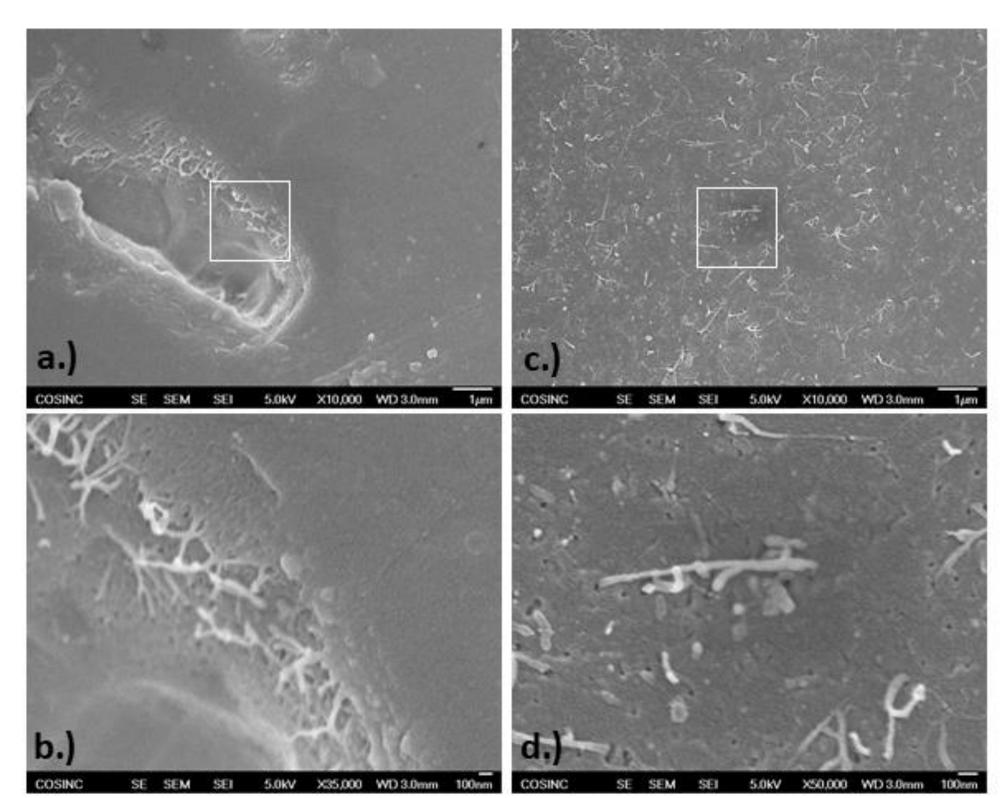
(a/b) PES\_U surface (bonded at 45min) presents a dense layer of PP with no visible open pores. (c) PES\_M surface (bonded at 45min) presents fiber-like at the pore interface (d). This image is verified using AFM (f) which clearly presents two different modulus values indicating two different materials: soft PP and rigid PES\_M.
