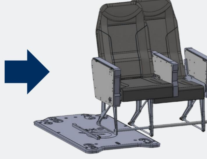
3. Lock in Place - Ensure the seat clicks and aligns flush on the far side
