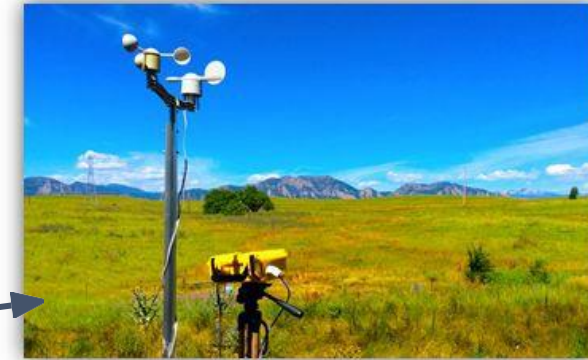
monitoring CH 4 and VOCs near gas facility
