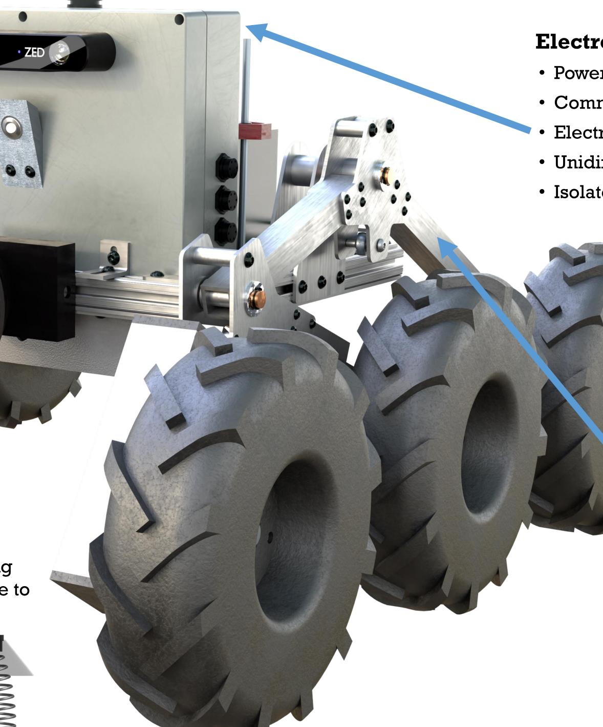
The Zed2i stereo camera allows the rover to capture the 3d geometry of the environment.
