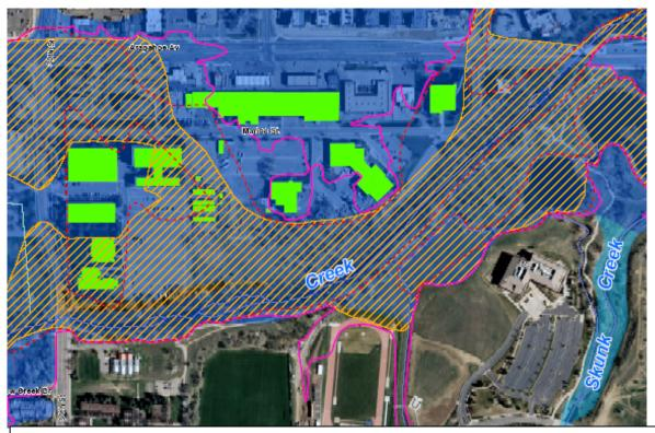
Figure 2.3: The flood plain mapping for a portion of Boulder Creek through the East Campus. The blue shaded area is the existing flood plain. The solid pink line is the proposed flood plain and the hatched area is the flood conveyance zone where structures should be avoided.
