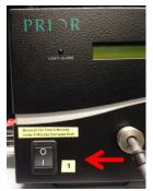
2) Turn on the Prior Proscan III stage controller. The power switch is in the back, bottom right corner.
