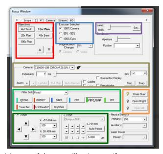
There is a **slider**, **called "Lamp"** that controls the brightness of the trans-illuminator. If you want to use trans-illumination, make sure that the condenser is in the down position and move the lamp slider to about 20% (you can adjust as needed, but this is a good starting position.) Then click on the "Brightfield" filter option and "Open Bright".
