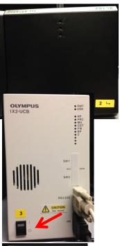
3) Turn on the Olympus IX2-UCB microscope controller power supply.
