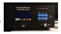
the stage (power, control, and gas), and turn on the gas as the control unit requires about 30 min to bring the system to 5% CO<sub>2</sub>. Leave the environmental stage outside of the microscope until it equilibrates to make sure the system does not leak into the microscope. Place an empty dish in the insert to partially seal the system and help it equilibrate faster. Once it is stable and at temp/CO<sub>2</sub>, place the unit on the microscope stage.
