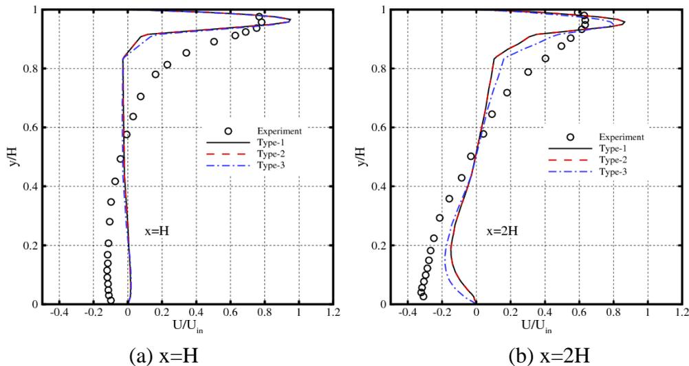
Fig.5 Compares of horizontal velocities of forced convection flow calculated by FFD with different time-splitting methods
