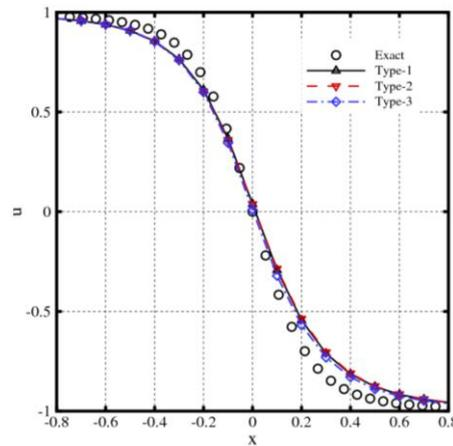
Fig.1 Comparison of Numerical Solution of Burgers' equation,  $t=2$
