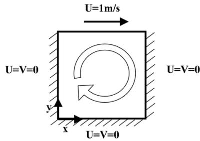
Fig.2 Schematic of Lid-Driven cavity flow
