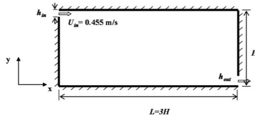
Fig.4 Schematic view of forced convection flow case
