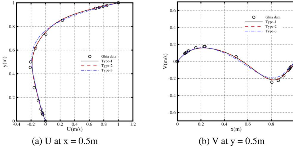
Fig.3 Comparison of horizontal and vertical velocities in a lid-driven cavity flow predicted by the FFD with different time-splitting methods. The reference data is high quality CFD data by Ghia et al. (1982).
