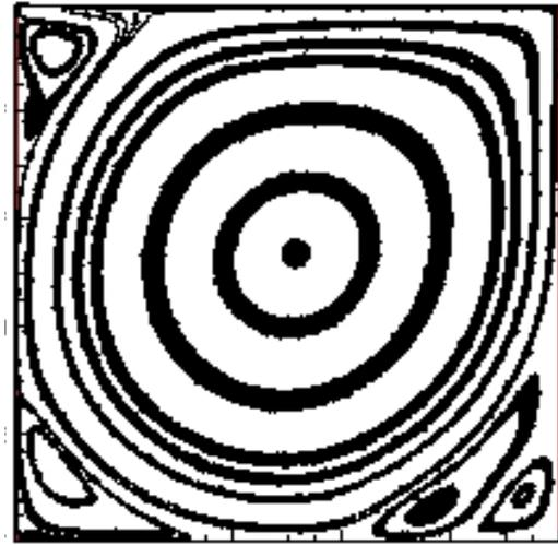
Figure 5 Streamlines of a turbulent lid-driven cavity flow ( $Re = 10000$ ) computed by the FFD on GPU
