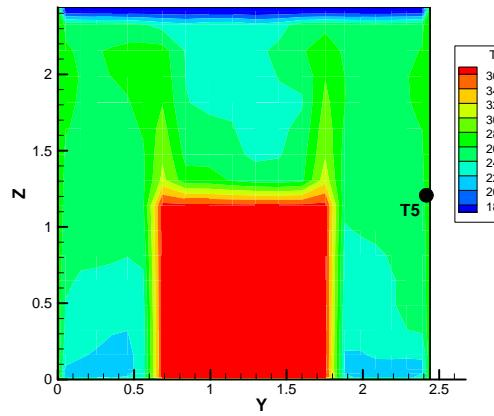
Figure 6 Temperature contour on a cross-section at  $X = 1.22$  m when thermostat is put at location 5
