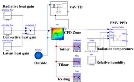
Figure 3. Modelica implementation of system model
