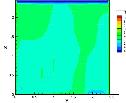
Figure 7 Temperature contour on a cross-section at  $X = 0.3$  m when thermostat is put at location 5
