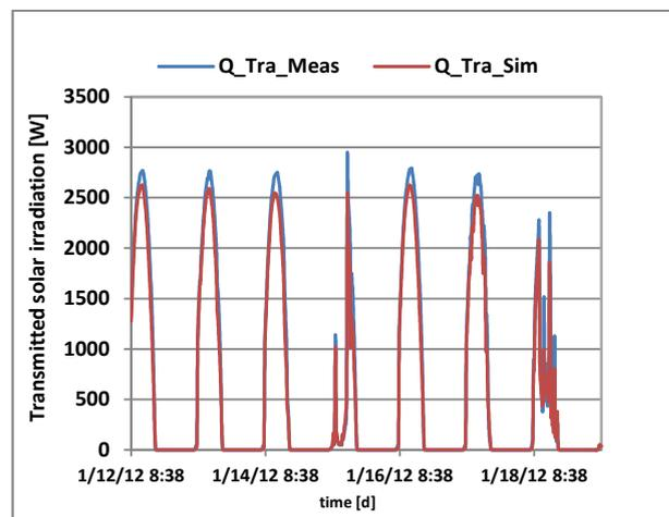
*Figure 13 Comparisons between simulated (red) and measured transmitted solar irradiations*
