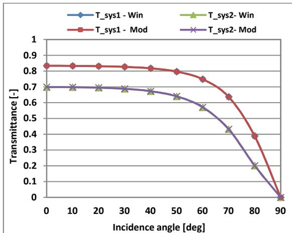
Figure 2 Transmittance values of single (sys1) and double pane (sys2) glazing systems calculated at different incidence angles using WINDOW 6 with spectrally averaged data and Modelica
