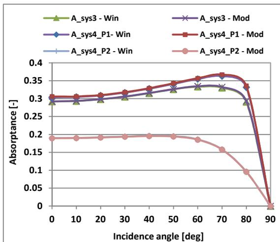
Figure 6 Absorbance values of single (sys3) and double pane (sys4) glazing systems calculated at different incidence angles using WINDOW 6 with spectrally averaged data and Modelica
