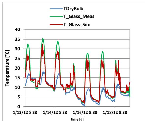
Figure 17 Comparisons between simulated and measured exterior pane outside surface temperature
