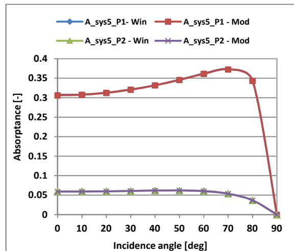
Figure 8 Absorbance values of double pane (sys5) glazing systems calculated at different incidence angles using WINDOW 6 with spectrally averaged data and Modelica
