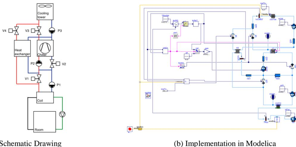
**Figure 1:** HVAC system with chilled water plant and water-side economizer.
