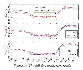
two methods. The prediction errors for the proposed method are within the range from  $-0.4^{\circ}C$  to  $0.5^{\circ}C$ . Those from the LSE method and the look-up table method are within the range from  $-1^{\circ}C$  to  $0.8^{\circ}C$ , and from  $-2^{\circ}C$  to  $-1^{\circ}C$ , respectively. Since the prediction on the occupied period is more important for implementing advanced building control, we believe the proposed method generates much better predictions.
