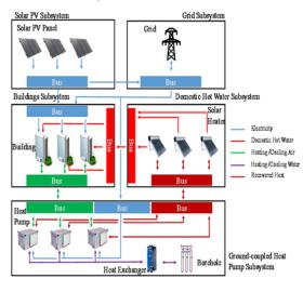
Figure 3 Block diagram for the exchange and communication of different subsystem models in NZEC
