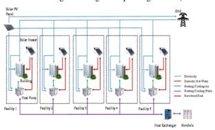
Figure 2 The schematic of the energy systems of HGV
