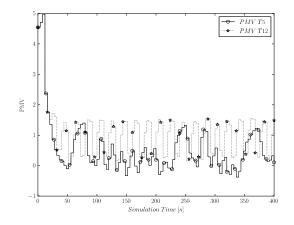
*Figure 9 PMV changing alone with time when* thermostat is put at location 5 and 12
