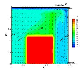
Figure 5 Temperature contour on a cross-section at Y = 1.22 m (Zuo et al. 2016)
