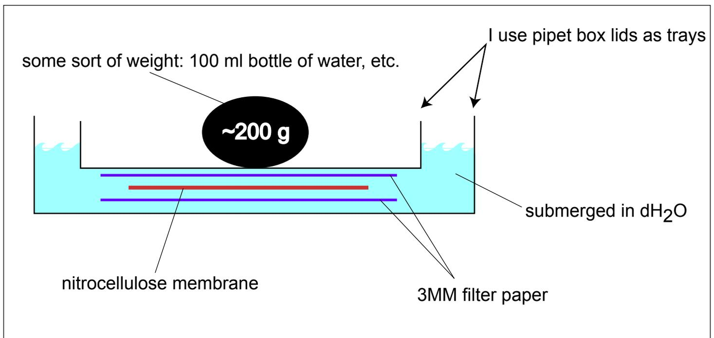
**Figure 1. Sandwiching blot for autoclaving**
