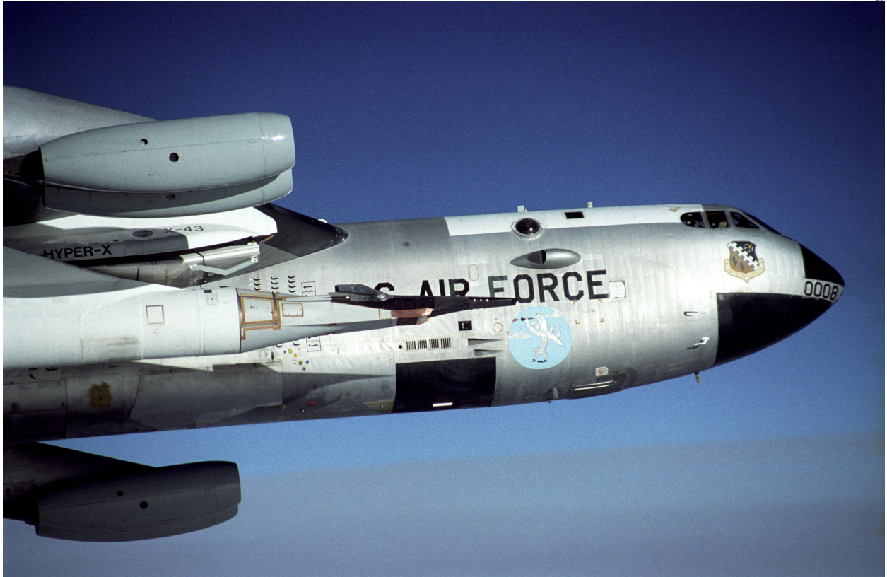
Figure 1.1: NASA X-43A scramjet attached to a Pegasus rocket being carried by a B-52. The B-52 took the X-43A/Pegasus assembly to 12 km altitude, where it would detach and climb using the rocket until the scramjet separated and ignited at approximately 30 km. This single image contains three of the most common combustion-based engines: 1) gas turbine engine (B-52), 2) rocket motor (Pegasus), and a 3) scramjet engine (X-43). [2]
