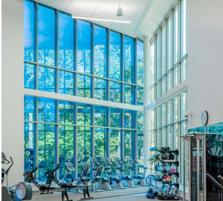
Electrochromic windows in Tarrytown, N.Y., USA, manufactured by View. The windows darken or lighten depending on where exactly the sun is shining. View Inc.
