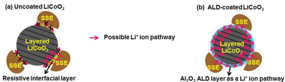
Figure 6. Schematic depiction of the interface between (a) uncoated LiCoO 2 & SSE, (b) Ar HT Al 2 O 3 ALD-coated LiCoO 2 & SSE.
