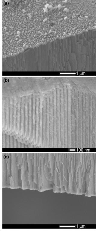
Fig. 3. Scanning electron micrographs of zircone-coated nanoporous alumina. (a) Cross section of the front side; pore features were not readily noted. (b) Cross section of the front side; some nanoparticles were noted within the pores. (c) Cross section of the back side; open pores were noted.
