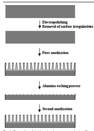
Fig. 1. Preparation of highly ordered nanoporous alumina. Reproduced from Ref. 19 with permission of The Royal Society of Chemistry.
