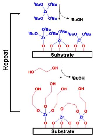
Fig. 2. Schematic depicting the growth of zircone MLD films using zirconium tert-butoxide and EG. Reproduced from Ref. 15 with permission of John Wiley & Sons, Inc.
