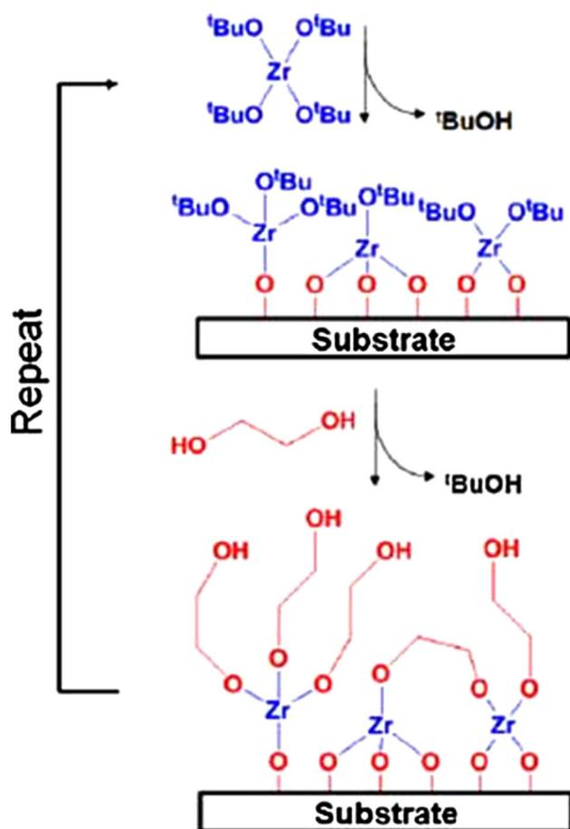
Fig. 2. Schematic depicting the growth of zirconium MLD films using zirconium tert-butoxide and EG. Reproduced from Ref. 15 with permission of John Wiley & Sons, Inc.
