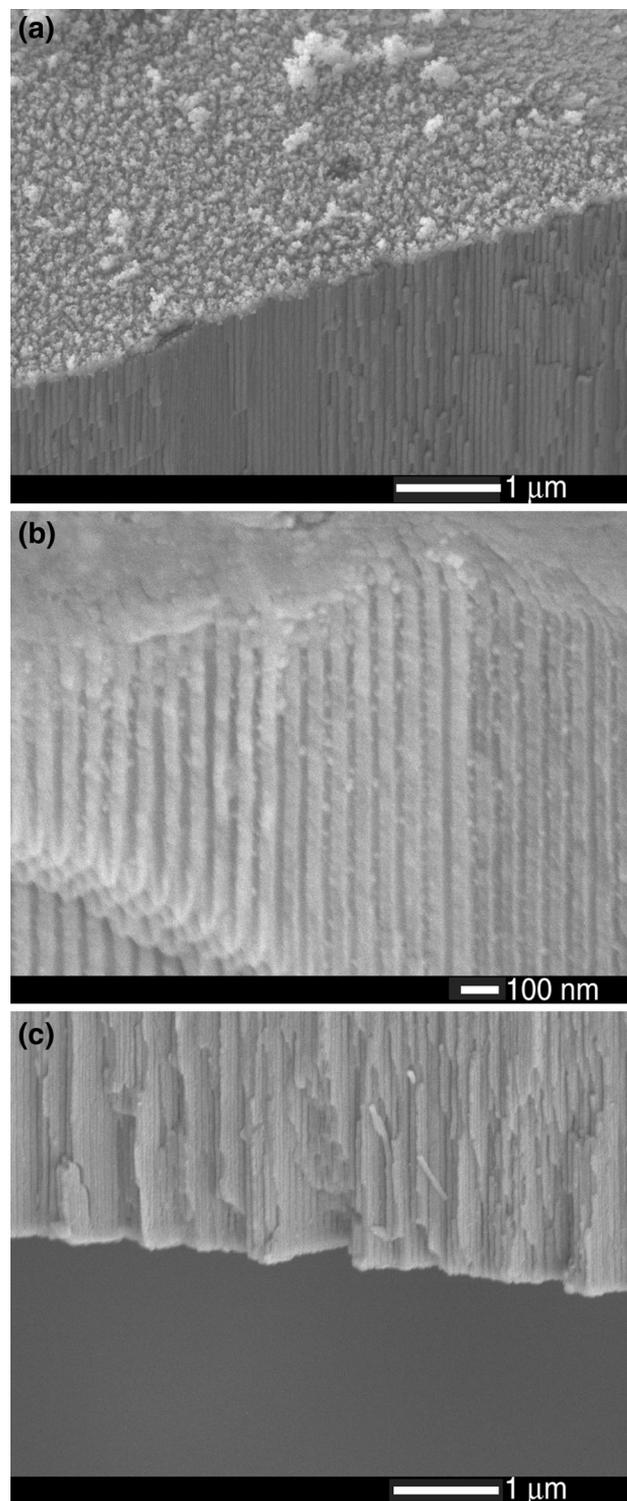
Fig. 3. Scanning electron micrographs of zirconium-coated nanoporous alumina. (a) Cross section of the front side; pore features were not readily noted. (b) Cross section of the front side; some nanoparticles were noted within the pores. (c) Cross section of the back side; open pores were noted.
