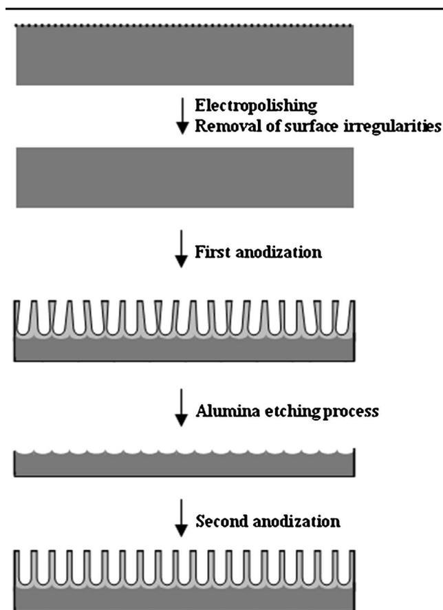
Fig. 1. Preparation of highly ordered nanoporous alumina. Reproduced from Ref. 19 with permission of The Royal Society of Chemistry.
