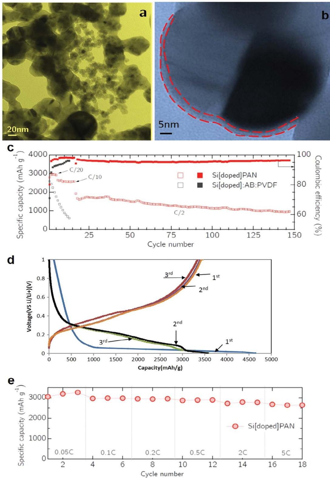
**Figure 1.** TEM of (a) silicon nanoparticle; (b) native oxide on silicon nanoparticles; (c) charge and discharge capacity of doped nano-Si/cyclized-PAN versus cycle number at C/20, C/10, and C/2 rate; (d) voltage profile of doped nano-Si/cyclized-PAN at C/20; (e) rate performance of doped nano-Si/cyclized-PAN.
