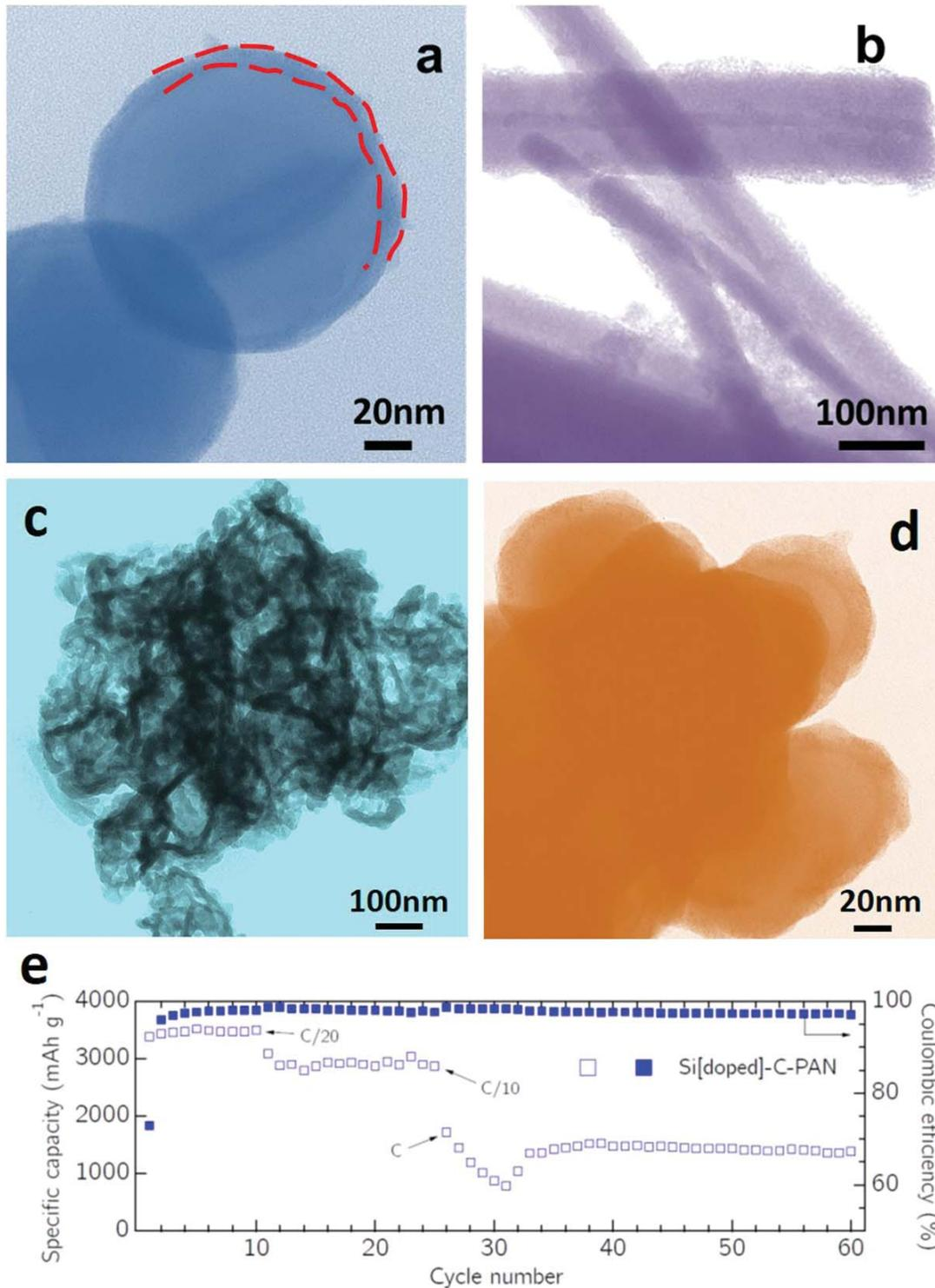
**Figure 2.** TEM of (a) carbon-coated silicon nanoparticle; (b) CNT found in carbon-coated silicon sample; (c) CNT embedded in nano-silicon/cyclized-PAN; (d) carbon coating remains on lithiated nano-silicon/cyclized-PAN; (e) discharge capacity of carbon-coated doped nano-Si/cyclized-PAN versus cycle number at C/20, C/10, and C rate.
