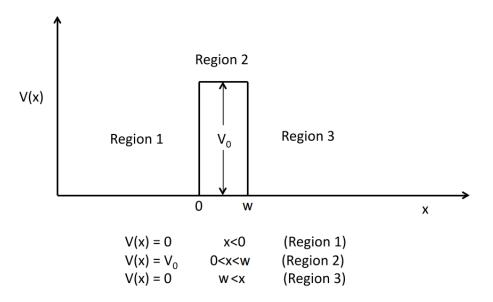
(a) We will find the wavefunction for the entire problem by finding a solution for each of the three regions and then "stitching" them together. Write down the time independent Schrödinger equation (TISE) for each of the three regions. Note that the energy of the particle is less than  $V_0$  (E <  $V_0$ ).
