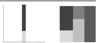
Stacked bar graph provides only length encoding because the bars' bases are misaligned. A treemap (Shneiderman, 1992) provides area encoding, which affords the least precise comparison of data values
