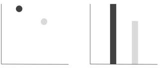
**Fig. 1** For a single-value comparison, dot plot provides encoding of data value by spatial position in the *y*-dimension. Bar graph provides both spatial position (top of the bar) and redundant encoding by bar's length.
