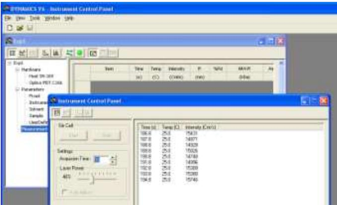
Values of around 150,000 to 600,000 cts/s are good. You can adjust the laser power to increase or decrease the values. Do not go below 10% laser power.
