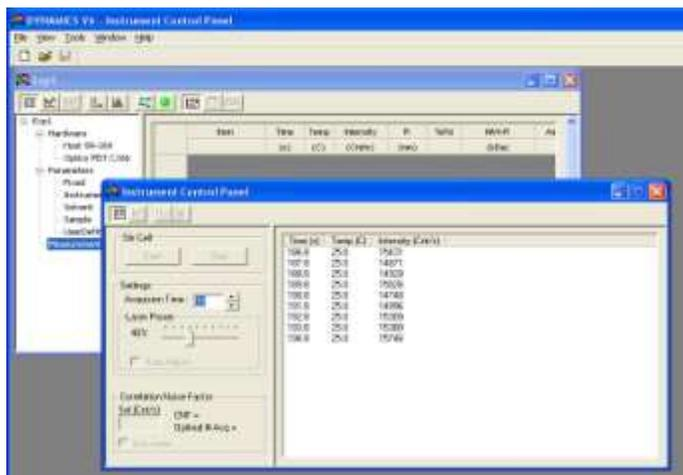
You can use this window to control laser power and acquisition time. Slowly increase laser power to 40%. **If the values are higher than 2,000,000 cts/s disconnect immediately, these readings are high enough that they can damage the detector (avalanche photodiode)!** A clean cuvette filled with filtered, bubble free  $\text{H}_2\text{O}$  should have readings between 15,000 and 20,000 cts/s.
