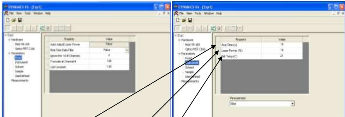
You can change AcqTime, Laser Power and Set Temp here. Good start values are Acq Time 10, Laser Power 10, and Set Temp (C) 21, they can be changed as required later.
