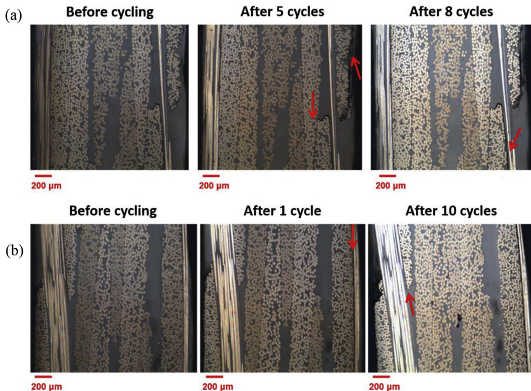
Fig. 11. a) Images taken before and after one and 10 hot cycles and b) Images taken before and after five and eight hot cycles.
